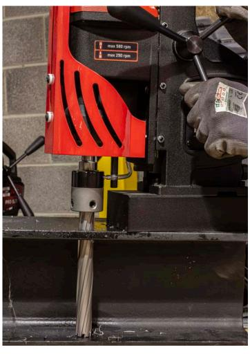
The 200mm TCT cutting length is perfect for reaching places you wouldn't be able to with a smaller cutter in a magdrill.
